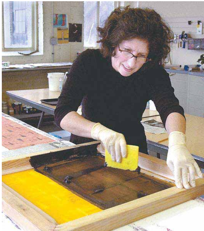
Laura Goldstein squeegees pigment on to fabric. She creates luxurious scarves through a painstaking process that includes hand-dyeing, silk-screening and as many as 30 cycles in a washing machine.
